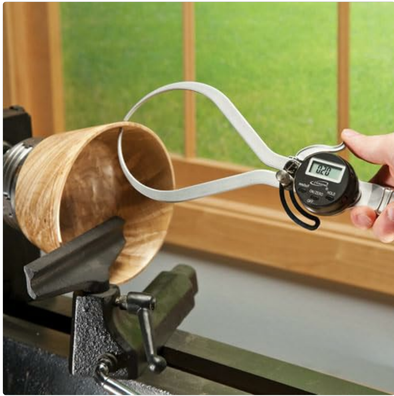
Image: A close-up view of the digital display and control buttons (mm/in/F, ON/SET, HOLD, OFF) on the caliper.
