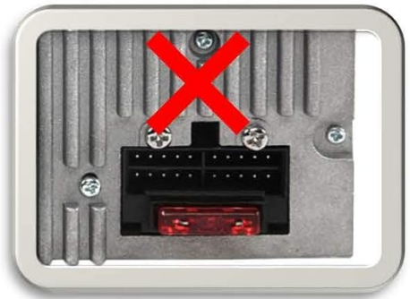
Image 2: Diagram illustrating compatible (ISO 8+8 Full pin) and incompatible (16 pin/20 pin) plug shapes for the wire harness.
