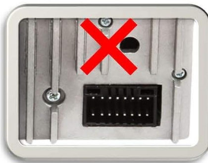
Image 2: Diagram illustrating compatible (ISO 8+8 Full pin) and incompatible (16 pin/20 pin) plug shapes for the wire harness.
