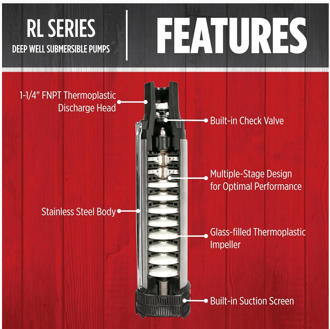
Image: Detailed diagram illustrating the internal features of the RL Series pump, including the 1-1/4" FNPT Thermoplastic Discharge Head, Built-in Check Valve, Multiple-Stage Design, Stainless Steel Body, Glass-filled Thermoplastic Impeller, and Built-in Suction Screen.
