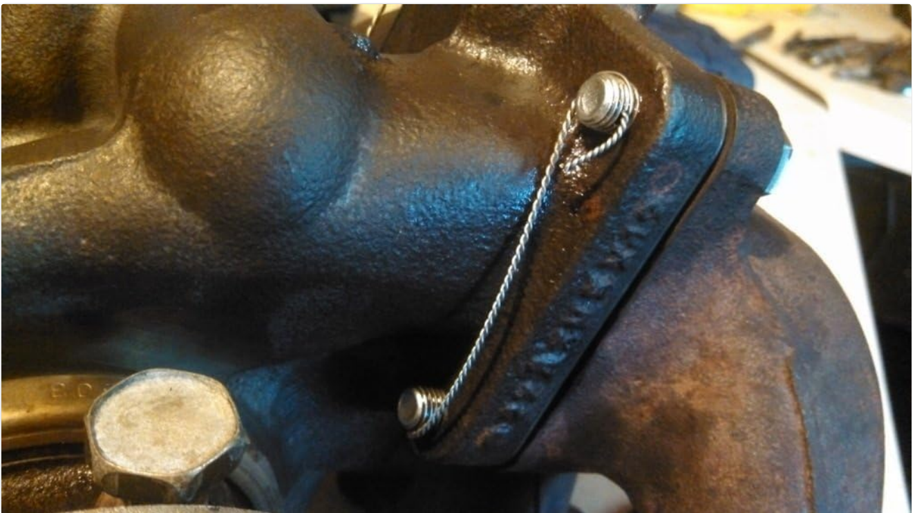
Image 3: An example of safety lock wire applied to secure bolts on an engine component. The wire is twisted between two bolts, preventing them from loosening.
