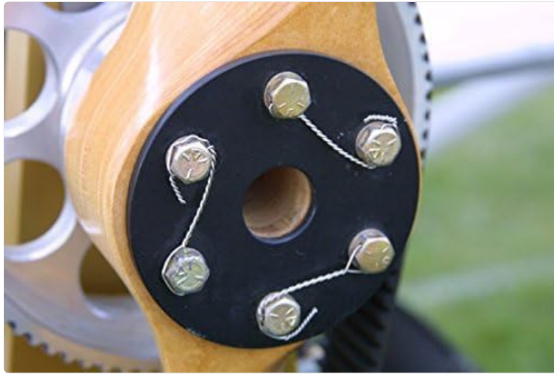
Image 4: Safety lock wire applied to secure multiple bolts on an aircraft propeller. This demonstrates a common application where multiple fasteners are secured in a series.
