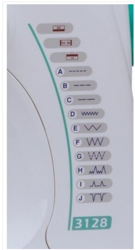
Figure 3: The stitch selection chart on the machine, displaying various stitch patterns labeled A through J.
