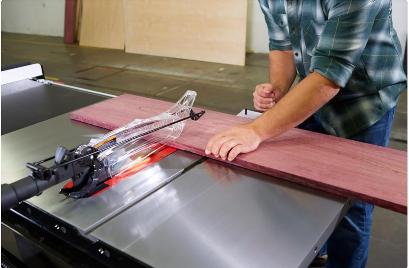
Figure 5: Demonstrating the blade guard in use during a cutting operation, effectively collecting dust.
