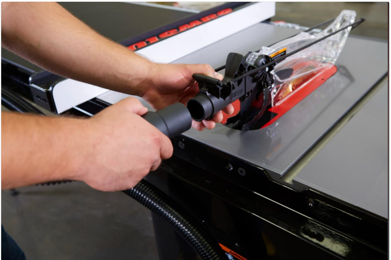
Figure 4: Connecting a dust collection hose to the integrated dust port on the blade guard.
