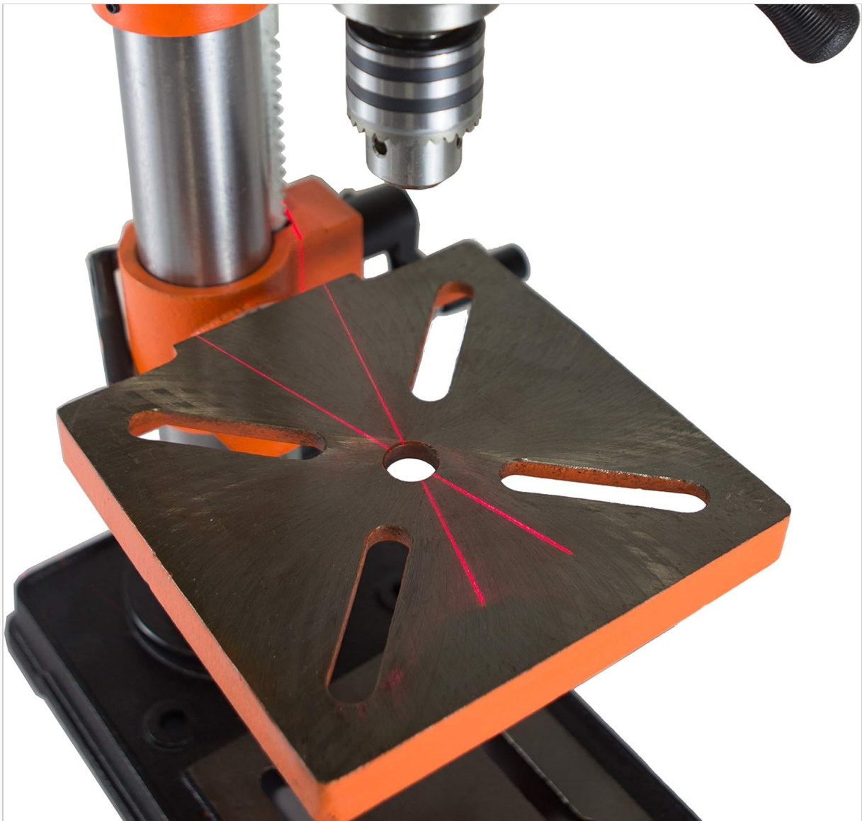
Figure 3: Laser centering device projecting an X-pattern on the worktable.
