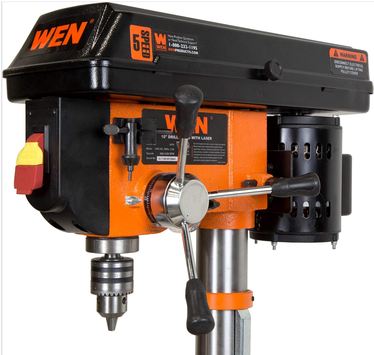
Figure 2: Control panel and pulley cover for speed adjustment.
