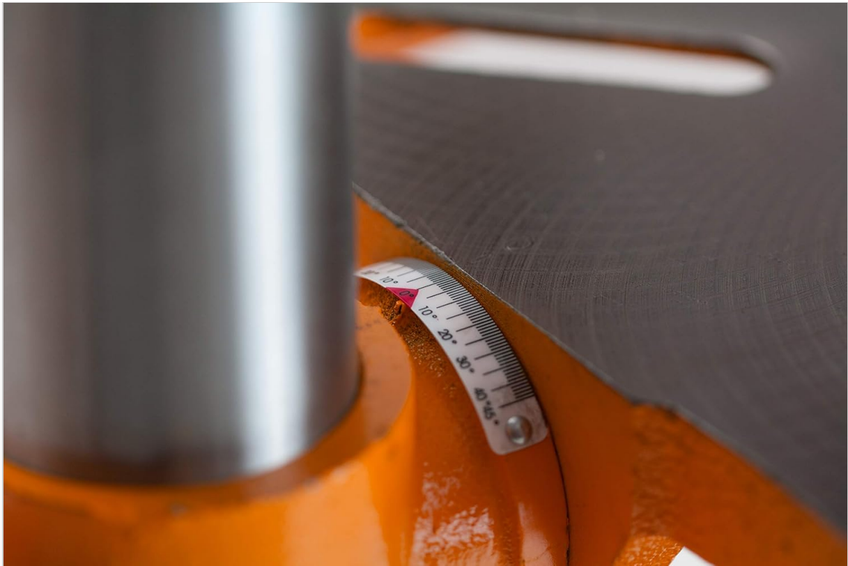
Figure 4: Worktable showing the bevel adjustment scale.
