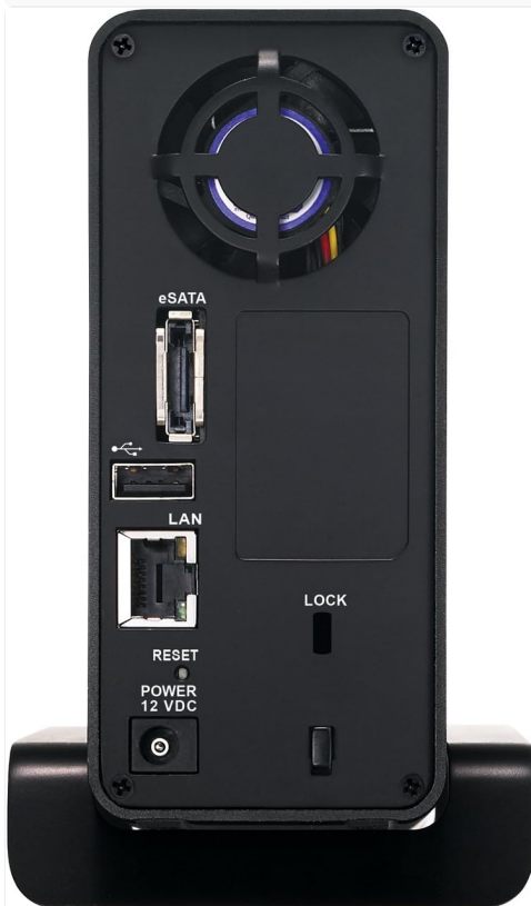
Figure 3: Angled view of the ZyXEL NSA310, providing a clearer perspective of the rear ports including eSATA, USB, LAN, and power input, along with the cooling fan.
