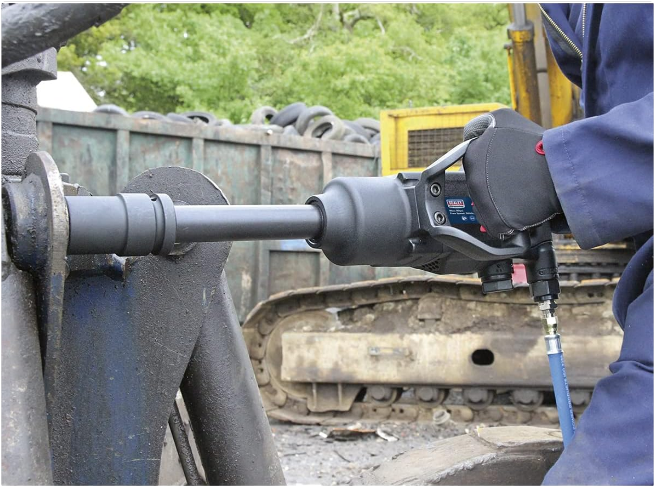
Figure 3: A side view of the impact wrench in operation, highlighting the extended anvil and the connection to the air hose.
