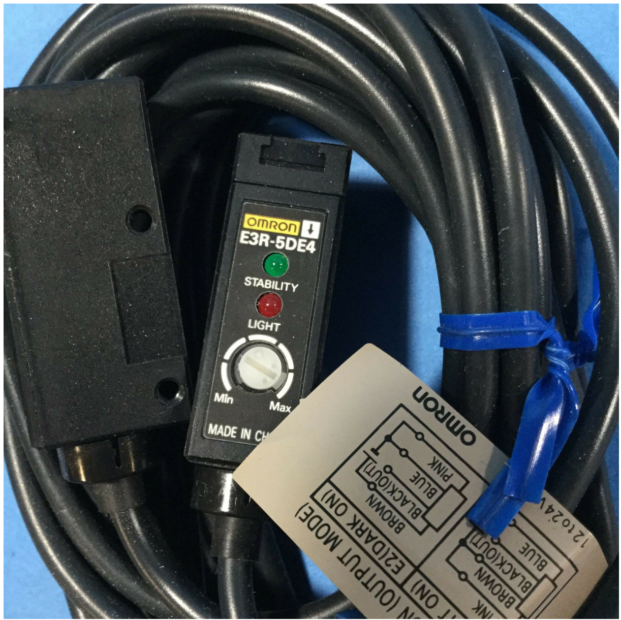
Figure 2: Detailed view of the E3R-5DE4 sensor, highlighting the sensitivity adjustment and the wiring diagram for connection.
