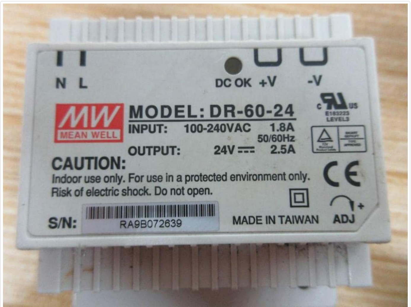
Figure 3.2: Close-up view of the top label on the DR-60-24, detailing input (100-240VAC, 1.8A) and output (24V, 2.5A) specifications, along with safety warnings and serial number.
