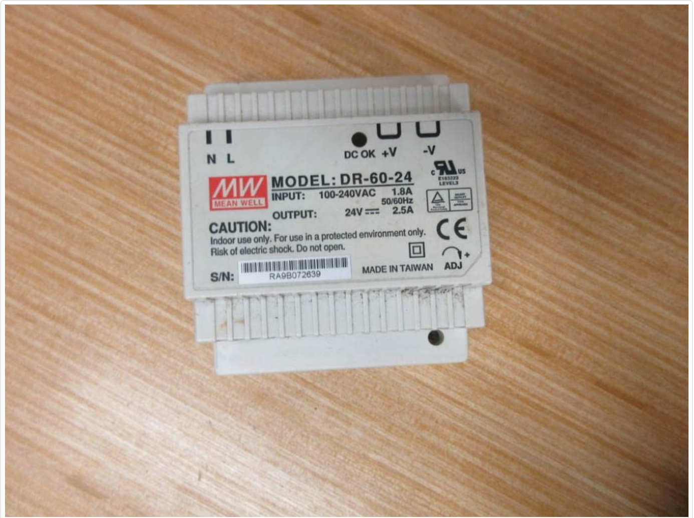
Figure 4.1: Top view of the DR-60-24, showing the terminal block layout and overall compact design suitable for DIN-Rail mounting.
