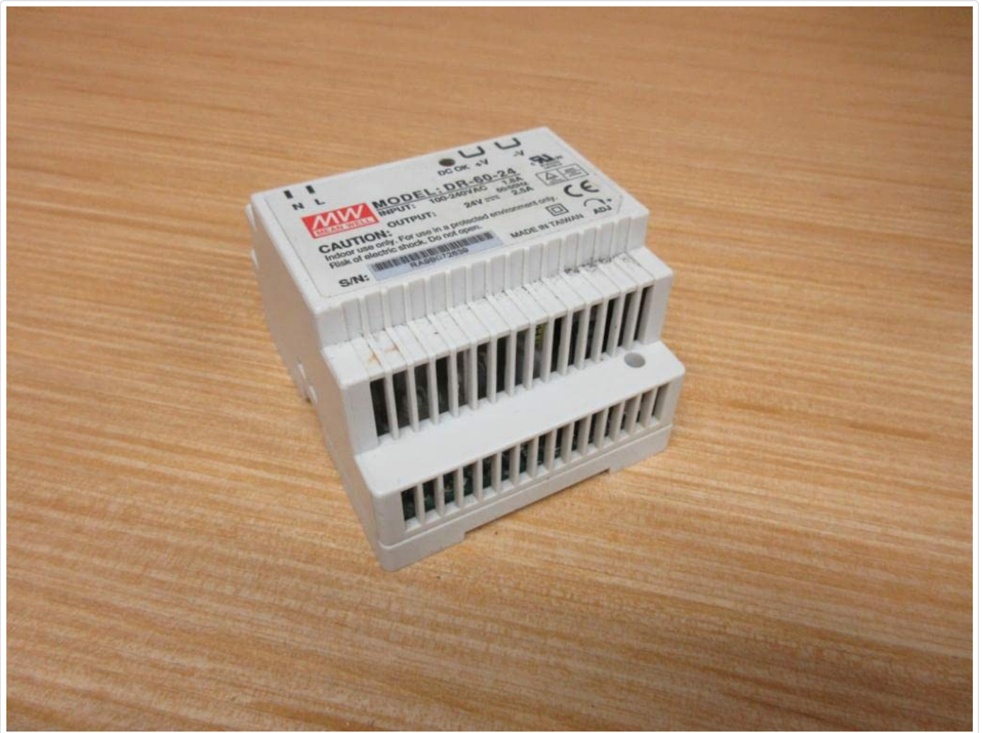
Figure 3.1: Front view of the Mean Well DR-60-24 power supply, showing the input/output terminals and model label.
