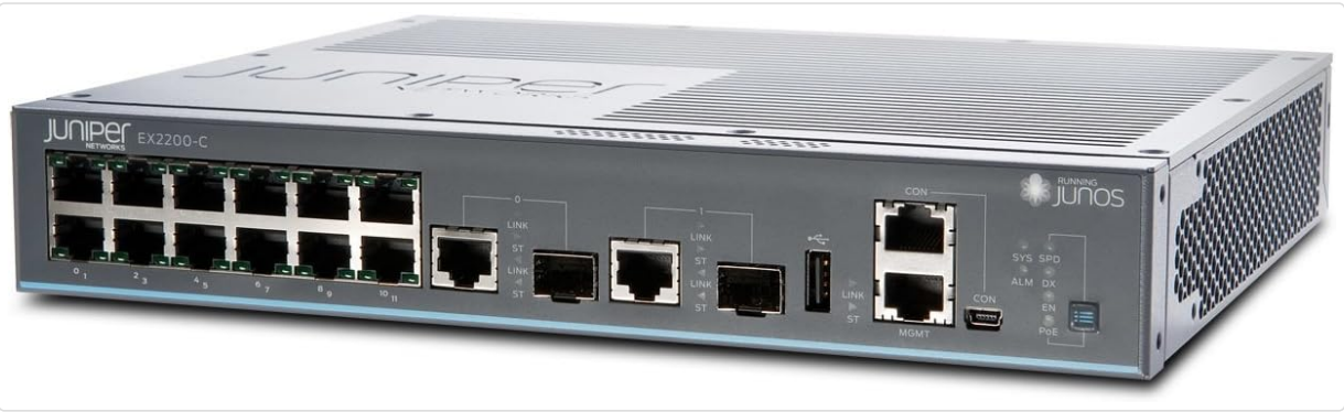
Figure 1: Front view of the Juniper EX2200-C-12T-2G Layer 3 Switch. This image displays the front panel of the switch, highlighting the 12 RJ-45 Ethernet ports, two SFP uplink ports, console ports (RJ45 and Mini-USB), and various status LEDs including SYS, SPD, ALM, DX, CON, EN, and PoE indicators.
