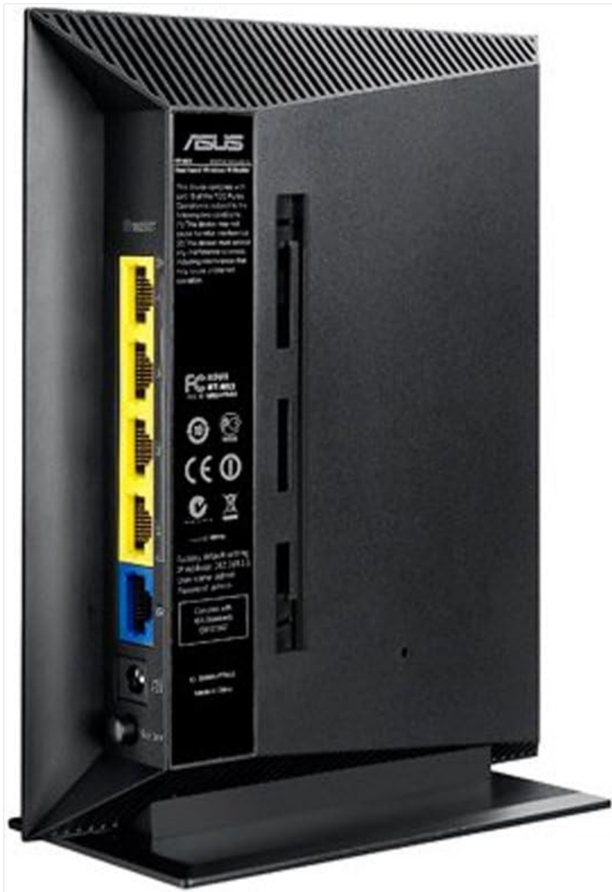
Figure 4: Back View with Product Information. This image displays the back of the ASUS RT-N53 router, showing the product label with model number, serial number, and regulatory compliance information. Mounting slots are also visible.
