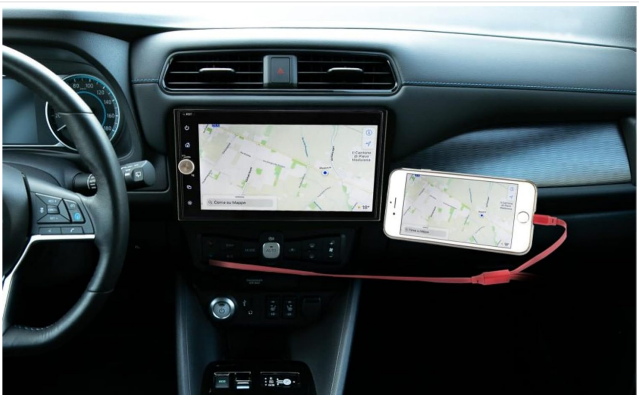
Image: The Phonocar VM060 multimedia system installed in a car dashboard, displaying a navigation map. A smartphone is connected via a red USB cable, mirroring the same navigation map onto its screen, demonstrating the Phonelink feature.
