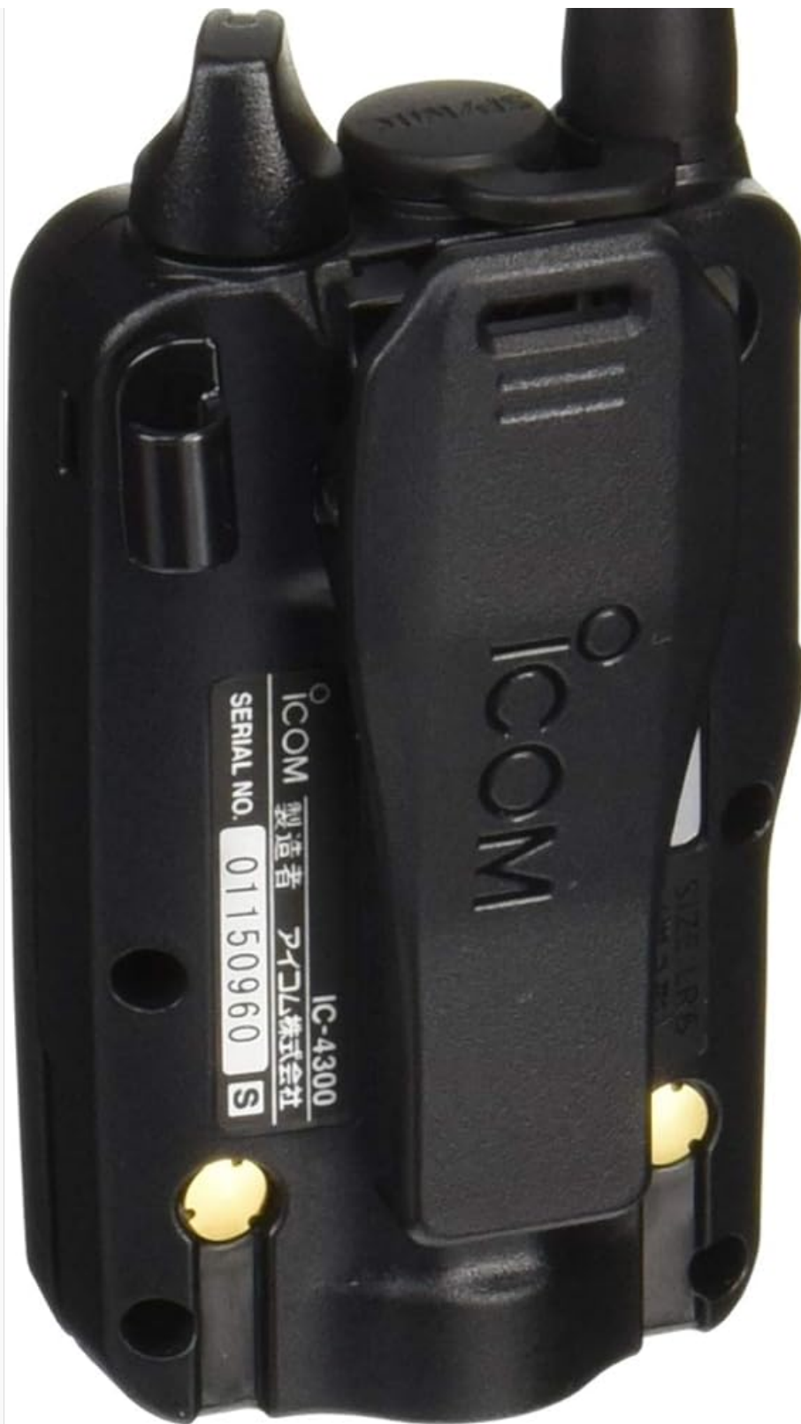
Figure 3.3: Back View. This image illustrates the rear of the ICOM IC-4300, featuring the removable belt clip and battery compartment cover.
