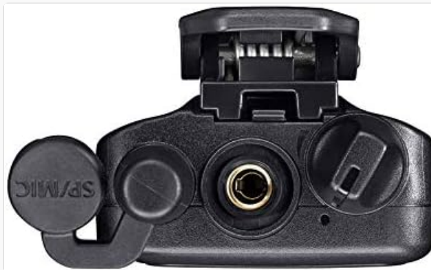
Figure 3.2: Top View. This image shows the top of the ICOM IC-4300, highlighting the covered speaker/microphone jack and the antenna connection point.
