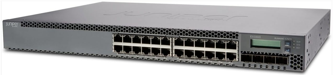
Figure 1: Front angled view of the Juniper EX3300-24T Ethernet Switch, showing the 24 Ethernet ports and four uplink ports.
