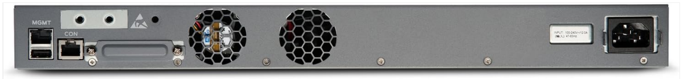
Figure 3: Rear view of the Juniper EX3300-24T Ethernet Switch, showing the power inlet, console port, and management port.
