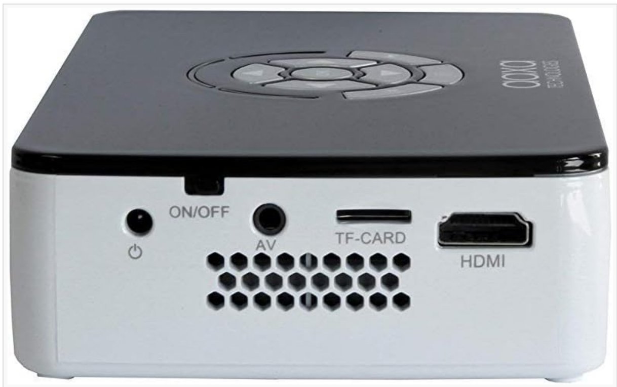
Figure 3.3: Right side panel, featuring the HDMI input, AV (composite) input, TF-CARD slot, and the power ON/OFF button.
