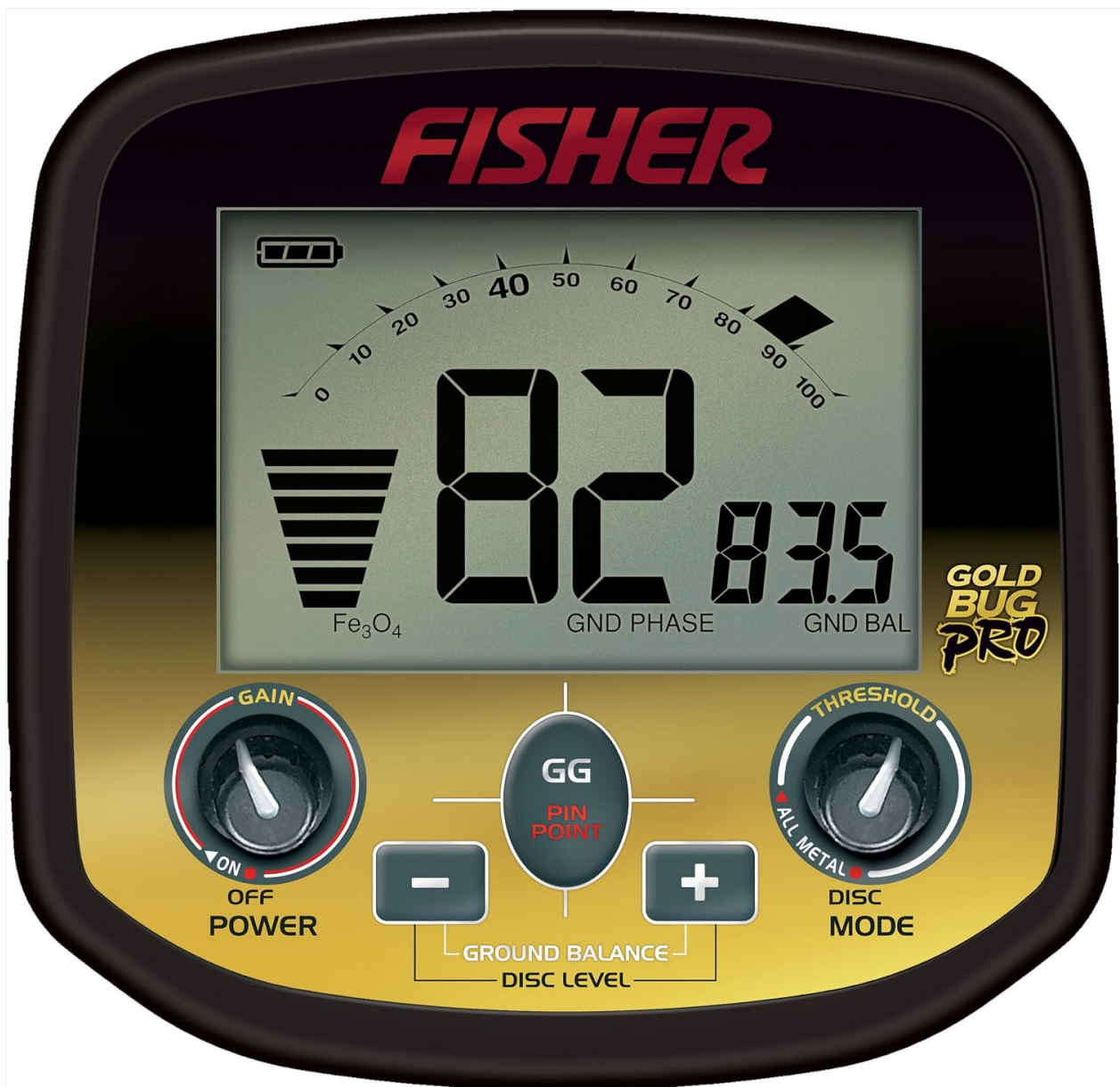
Figure 3.1: Close-up of the Gold Bug Pro control panel.
