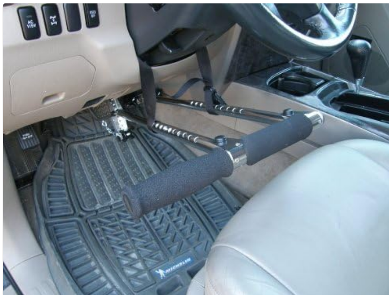
Image: A close-up view of the Freedom Staff 2.0 Hand Controls installed in the footwell of a vehicle, showing its connection to the pedals.
