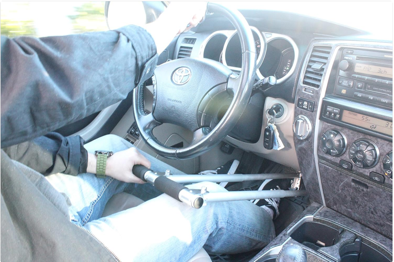
Image: A driver demonstrating the use of the Freedom Staff 2.0 Hand Controls, with one hand on the control lever and the other on the steering wheel.
