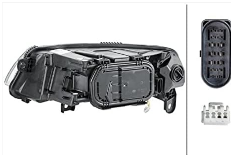
Figure 3.2: Rear view of the Hella 1EL 009 925-521 Bi-Xenon Headlamp, illustrating the housing and electrical connection points.
