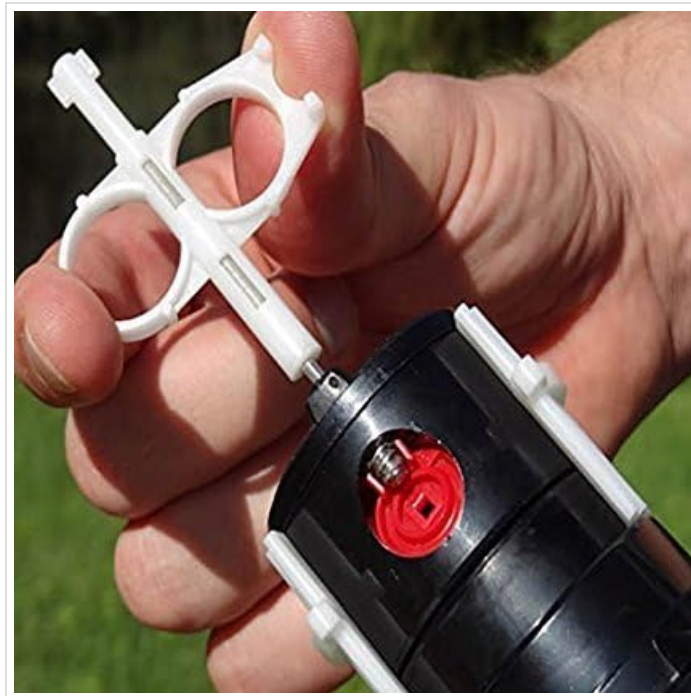
Figure 2: The Hunter adjustment tool being inserted into the top of a sprinkler head. The tool's key-like end fits into the designated adjustment slot on the sprinkler rotor.
