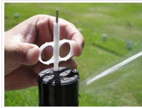
Figure 3: A hand holding the Hunter adjustment tool, which is inserted into a sprinkler head. Water is visibly spraying from the sprinkler, indicating an active system during adjustment.
