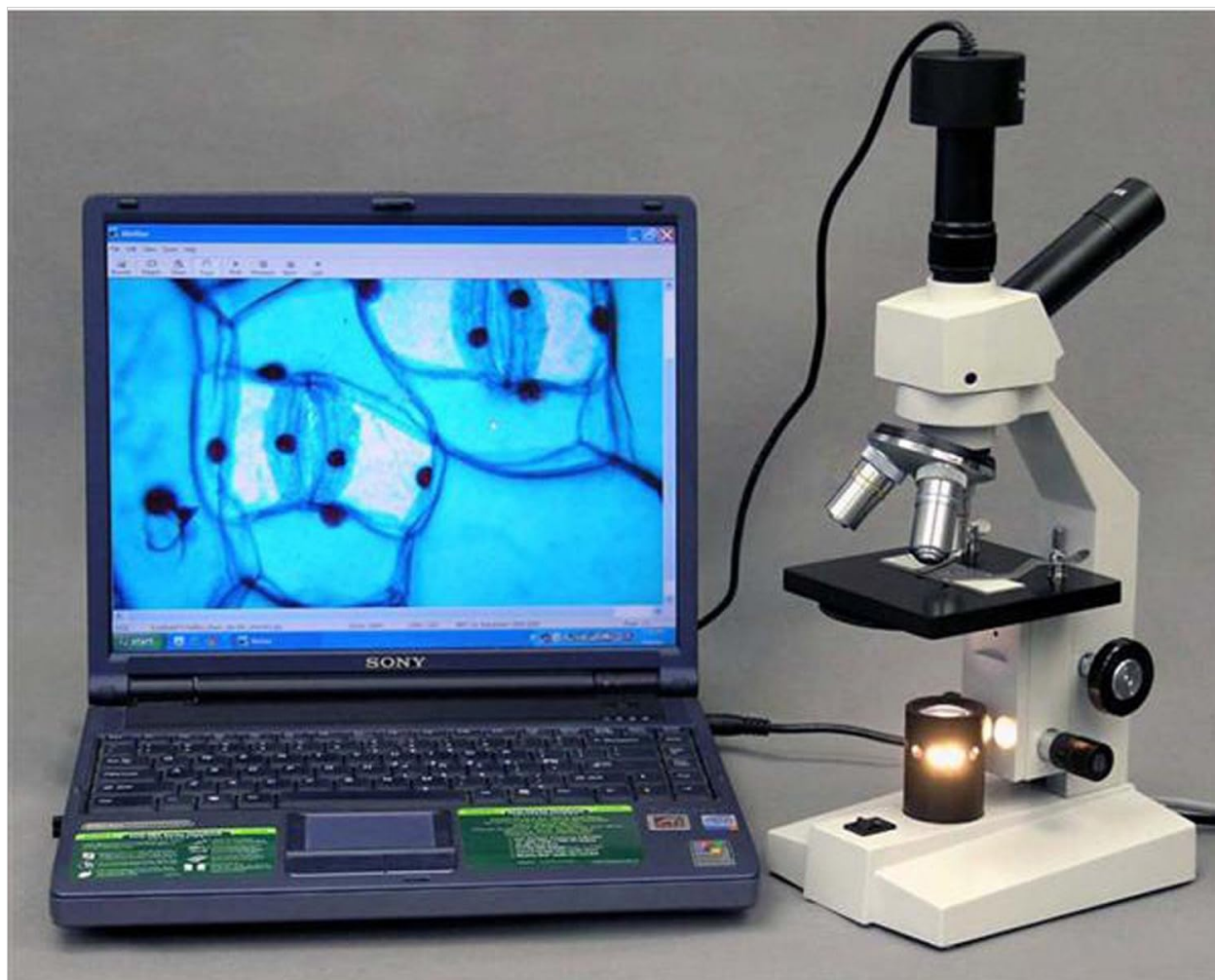
Figure 6.1: The AmScope D120A-MS microscope demonstrating its digital image capture capability by connecting to a laptop. This setup utilizes the vertical port for a camera attachment.
