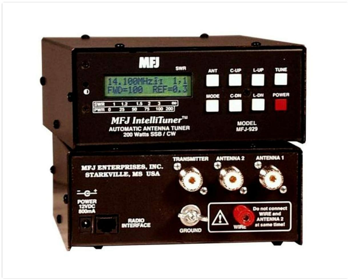
Figure 1: MFJ-929 IntelliTuner Front and Rear Panels. The top unit features a front panel with an LCD showing frequency, SWR, forward, and reflected power. Control buttons include ANT, C-UP, L-UP, TUNE, MODE, C-DN, L-DN, and POWER. The bottom unit shows the rear panel connections: 12VDC power input, Radio Interface port, Transmitter output, Antenna 2 input, Antenna 1 input, Ground terminal, and a Wire antenna terminal with a warning not to connect Wire and Antenna 2 simultaneously.
