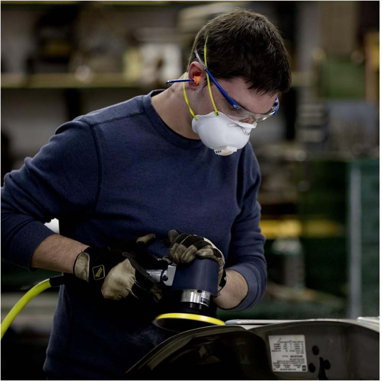
Figure 3: A user operating an air-powered sander, demonstrating a common application for this air compressor in workshops for surface preparation and finishing tasks.
