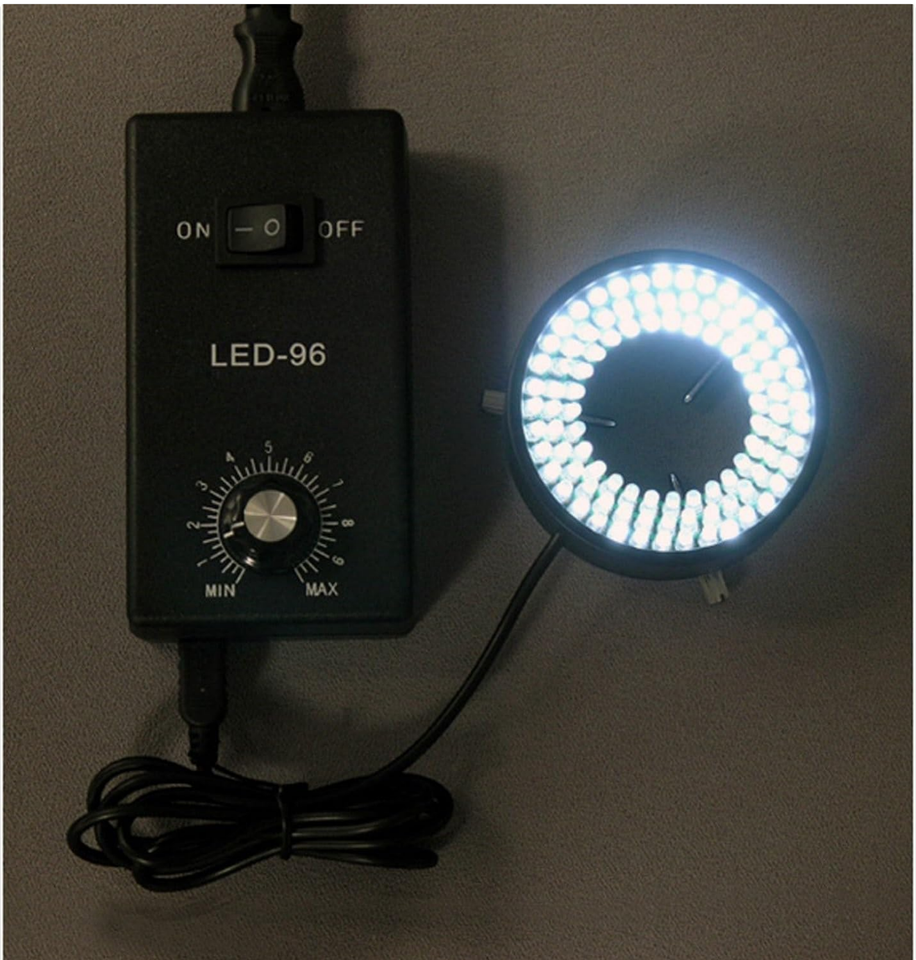
Figure 2: The 96-LED ring light connected to the control box.
