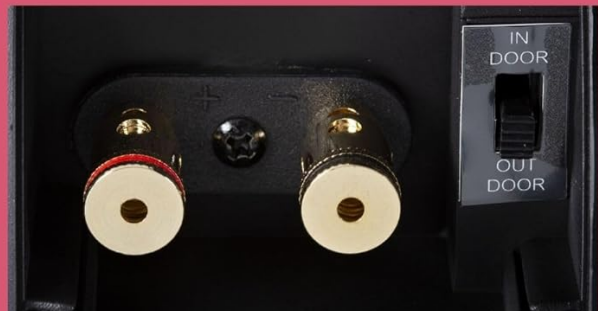
Image: The back panel of the speaker, illustrating the gold-plated connectors and the indoor/outdoor mode switch.
