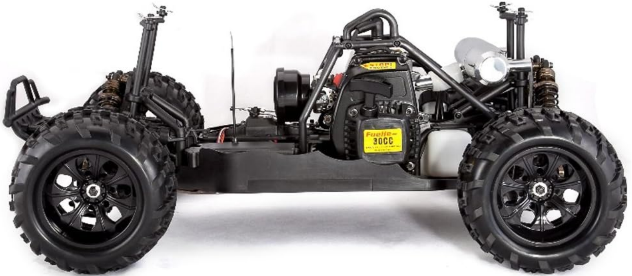
Figure 5.1: Top-down view of the Rampage XT chassis, revealing the engine, exhaust, fuel tank, and drivetrain components. This perspective is useful for maintenance and inspection.
