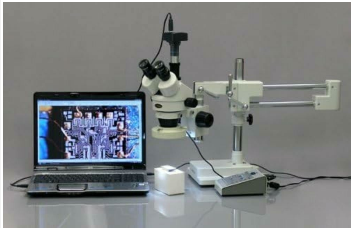
Image: The AmScope MU500-CK camera mounted on a stereo microscope, connected via USB to a laptop displaying a live image.
