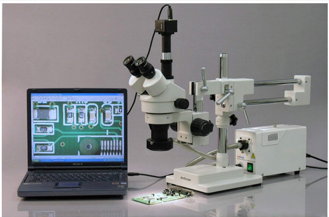
Figure 4.1: AmScope SM-4TPZ microscope connected to a laptop via the trinocular port for digital viewing. This setup demonstrates the capability to capture and display magnified images on an external screen, useful for documentation or collaborative viewing.
