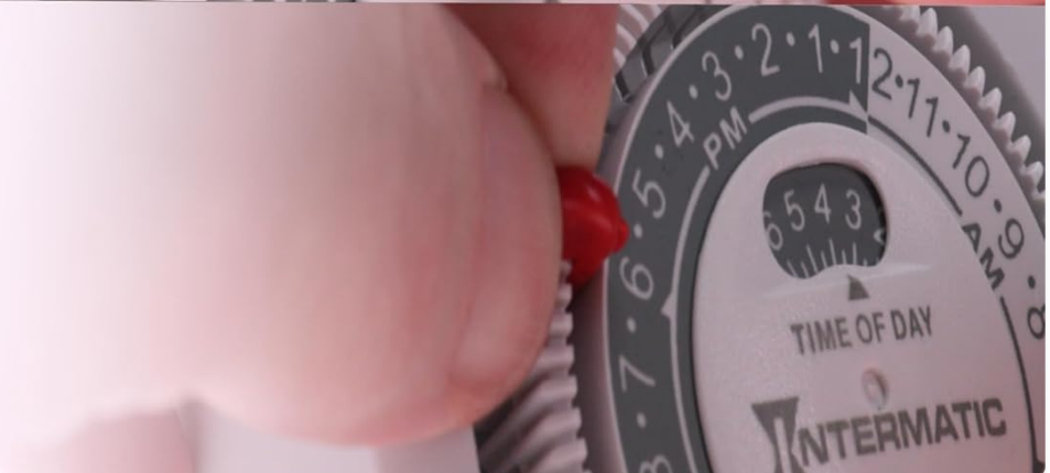
Figure 2.1: Visual guide for setting the time and inserting ON/OFF trippers.
