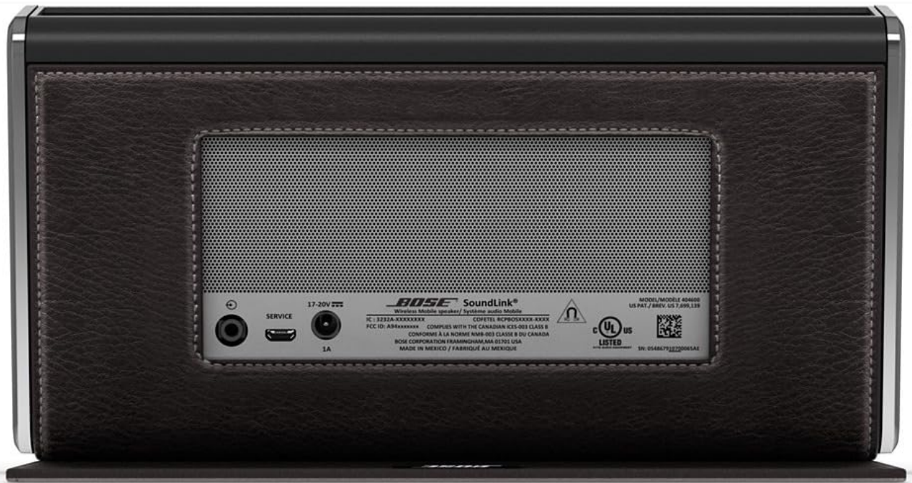
Figure 3: Rear ports including power, service, and AUX input.
