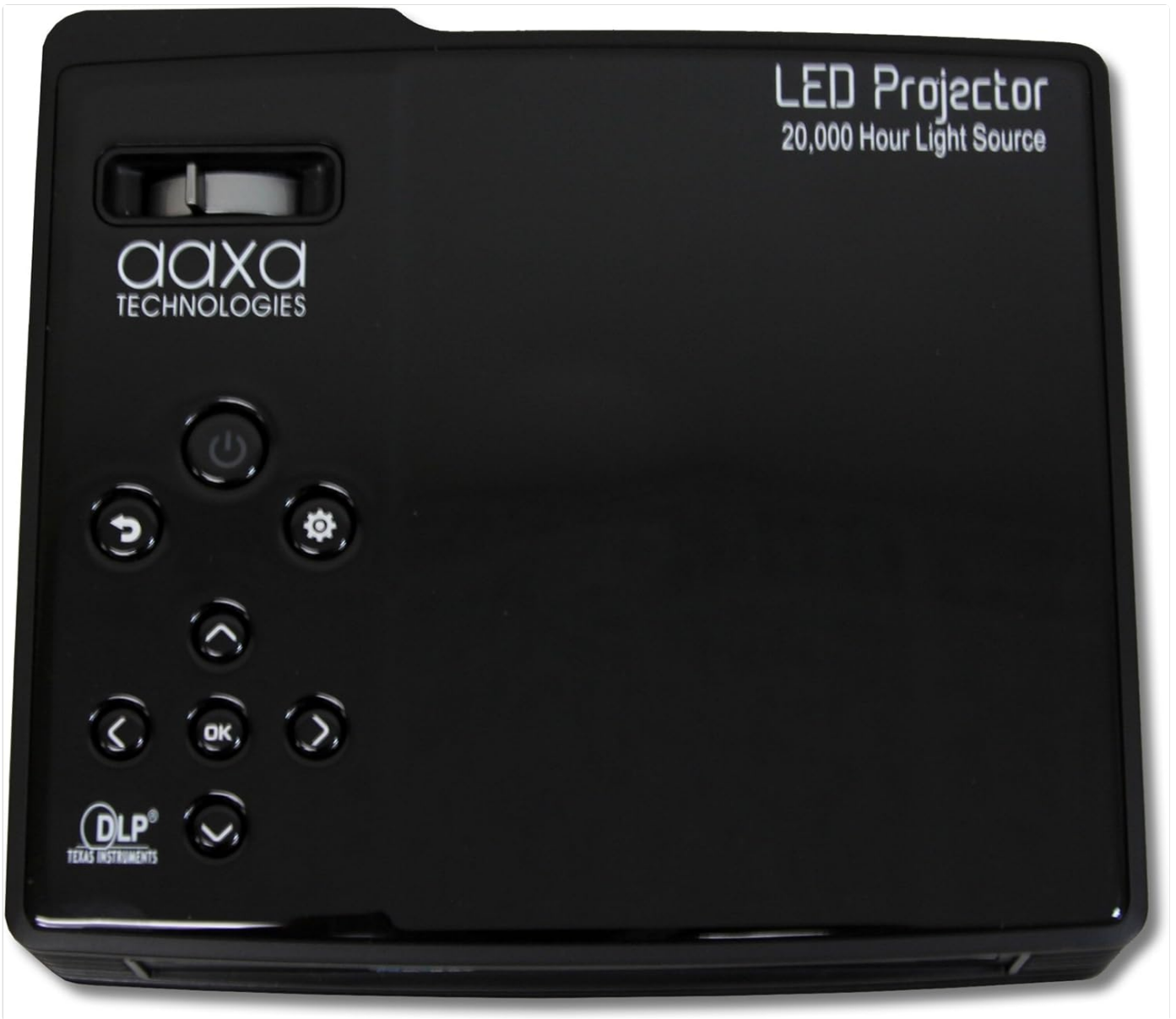
Figure 2: Top view of the AAXA MP-300-02 Projector, showing the integrated control panel.
