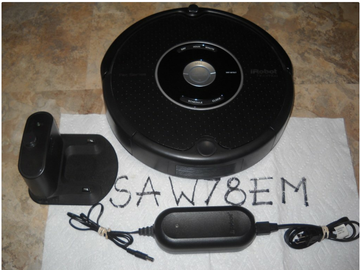
Image 1.1: The iRobot Roomba 552 Pet Series robotic vacuum, its Home Base charging station, and a Virtual Wall barrier device. The Roomba features a central control panel with 'CLEAN', 'SPOT', 'CLOCK', 'SCHEDULE', 'DAY', 'HOUR', and 'MINUTE' buttons. The Home Base is connected via a power cord.
