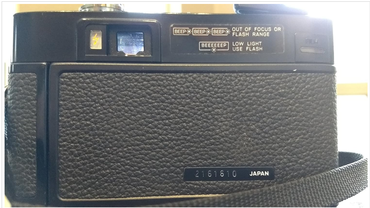
Figure 3: Back View. This image illustrates the back of the Minolta Hi-Matic AF2 camera, including the viewfinder, film counter, and indicators for out-of-focus/flash range and low light conditions.
