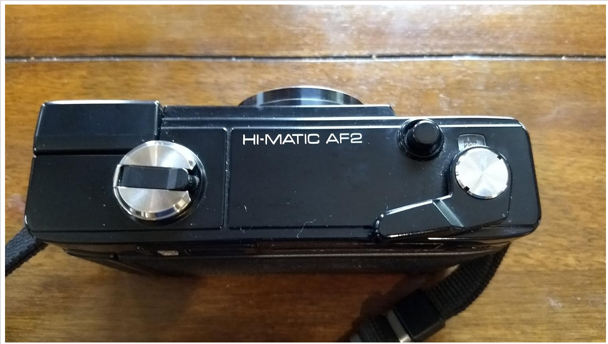
Figure 2: Top View. This image shows the top of the Minolta Hi-Matic AF2 camera, featuring the film advance lever, shutter button, and the camera's model name.
