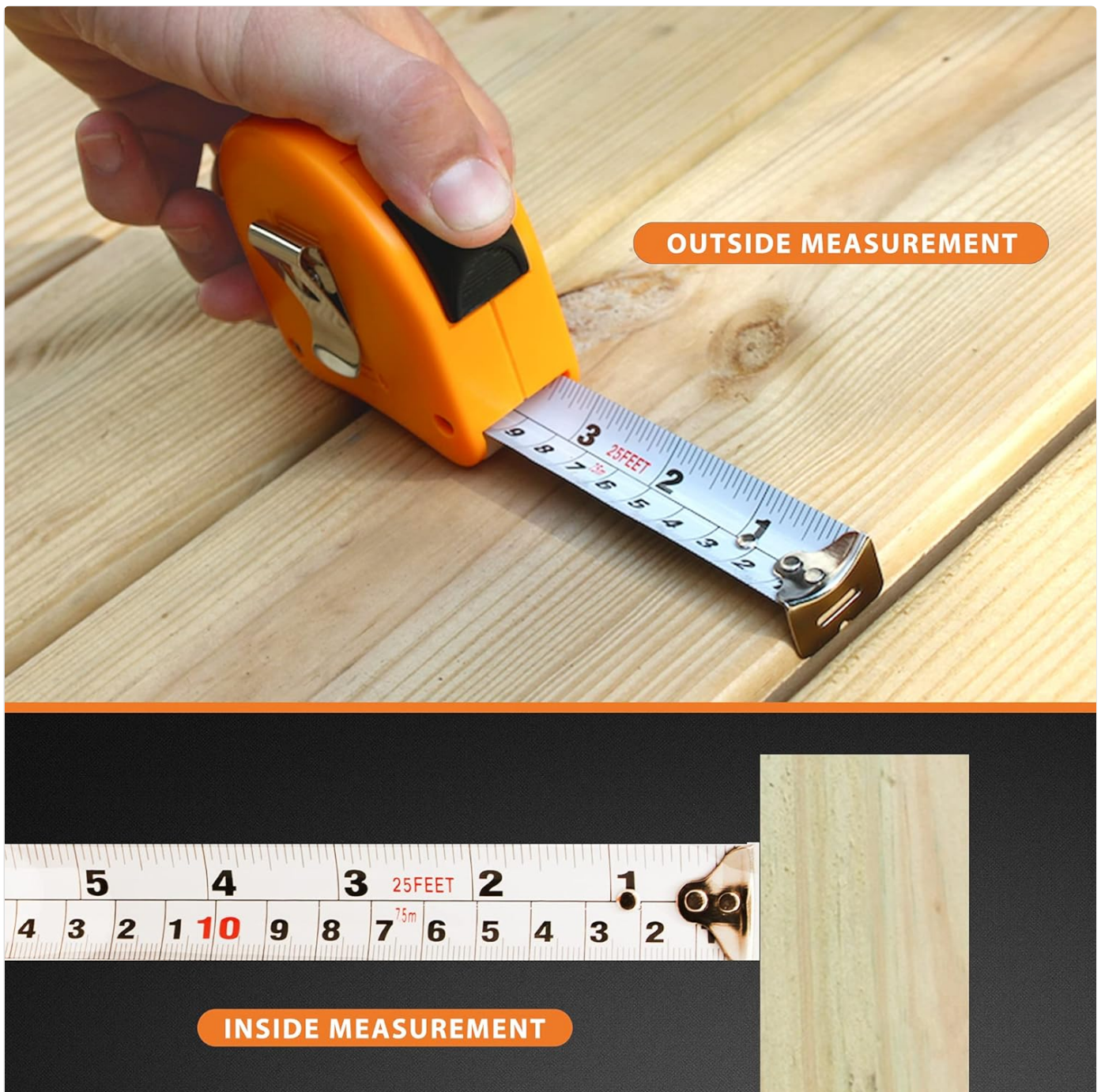
Figure 3.2: Demonstrates how to perform both outside and inside measurements using the tape measure, highlighting the correct placement of the end hook and tape case.
