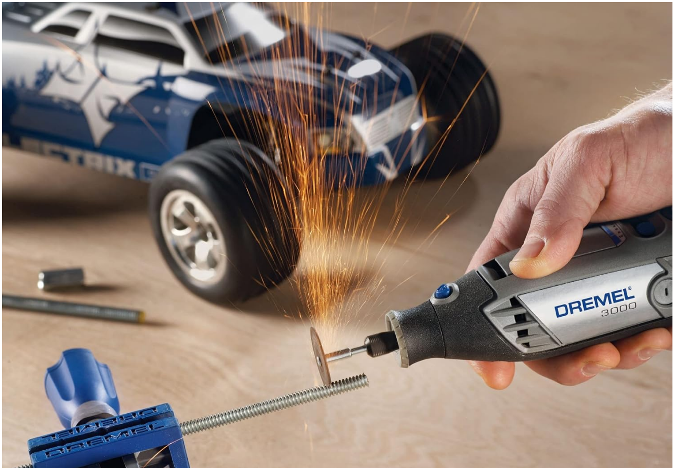
Image: The Dremel 3000 in use, cutting a metal rod, demonstrating its capability for precise metalwork.
