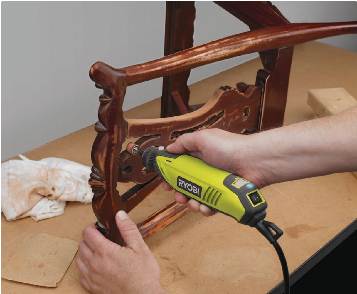
Figure 9: An example of the tool being used for sanding or polishing intricate wooden details.
