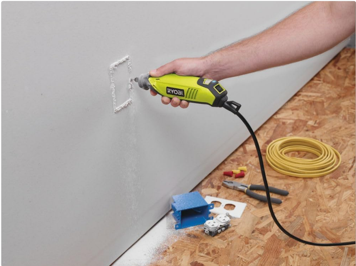
Figure 7: Using the rotary tool for cutting applications, such as creating openings in drywall.
