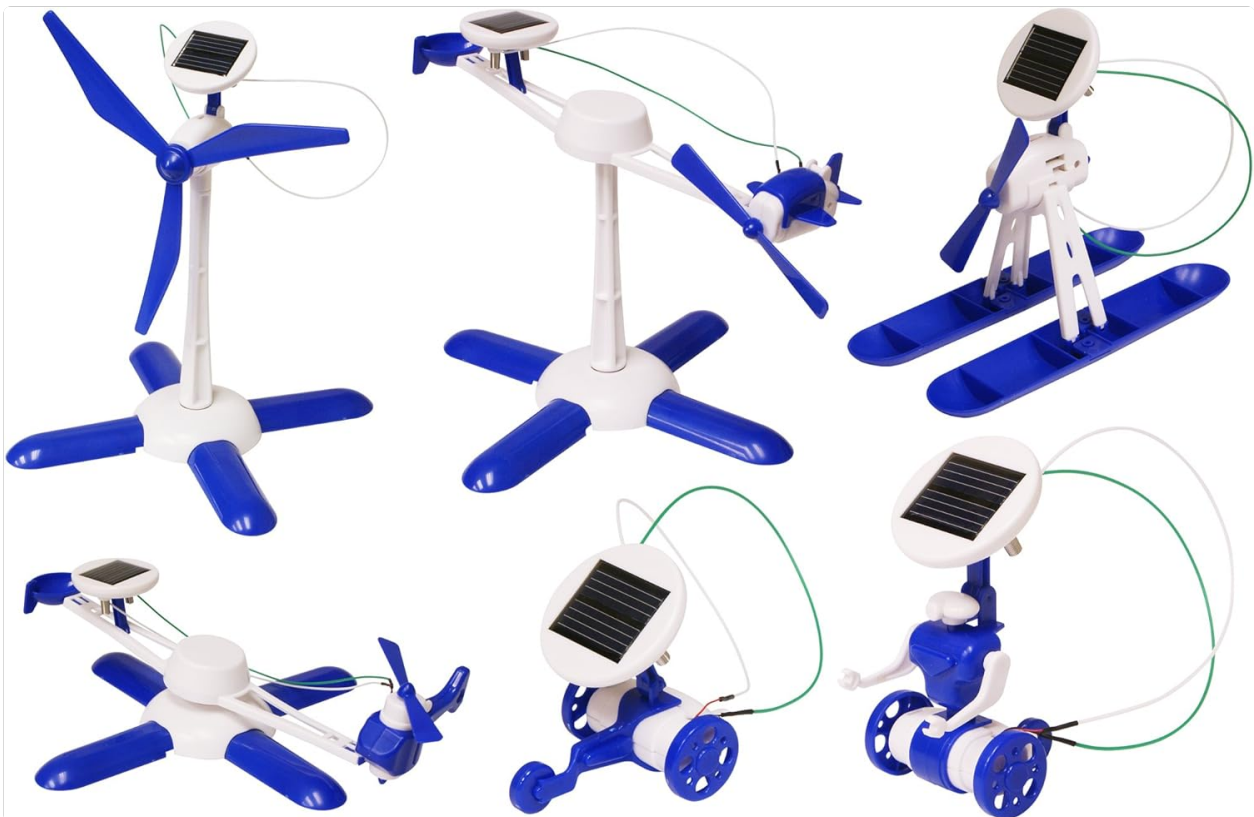
Figure 1: Overview of the six distinct models that can be constructed with the Edu-Toys 6-in-1 Solar Kit.
