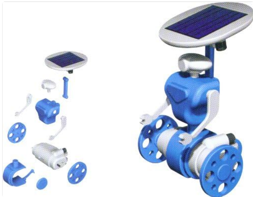
Figure 5: Assembly stages for the Solar Robot, detailing the body, wheels, motor, and solar panel components.
