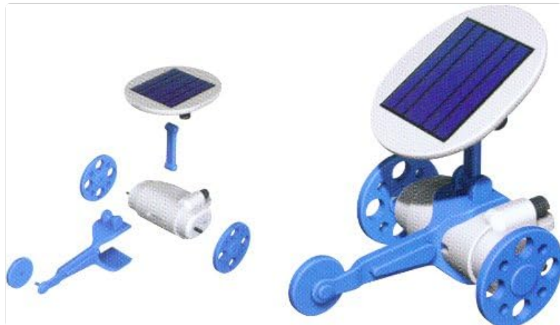
Figure 6: Assembly stages for the Solar Wheeler, showing the chassis, three wheels, motor, and solar panel.
