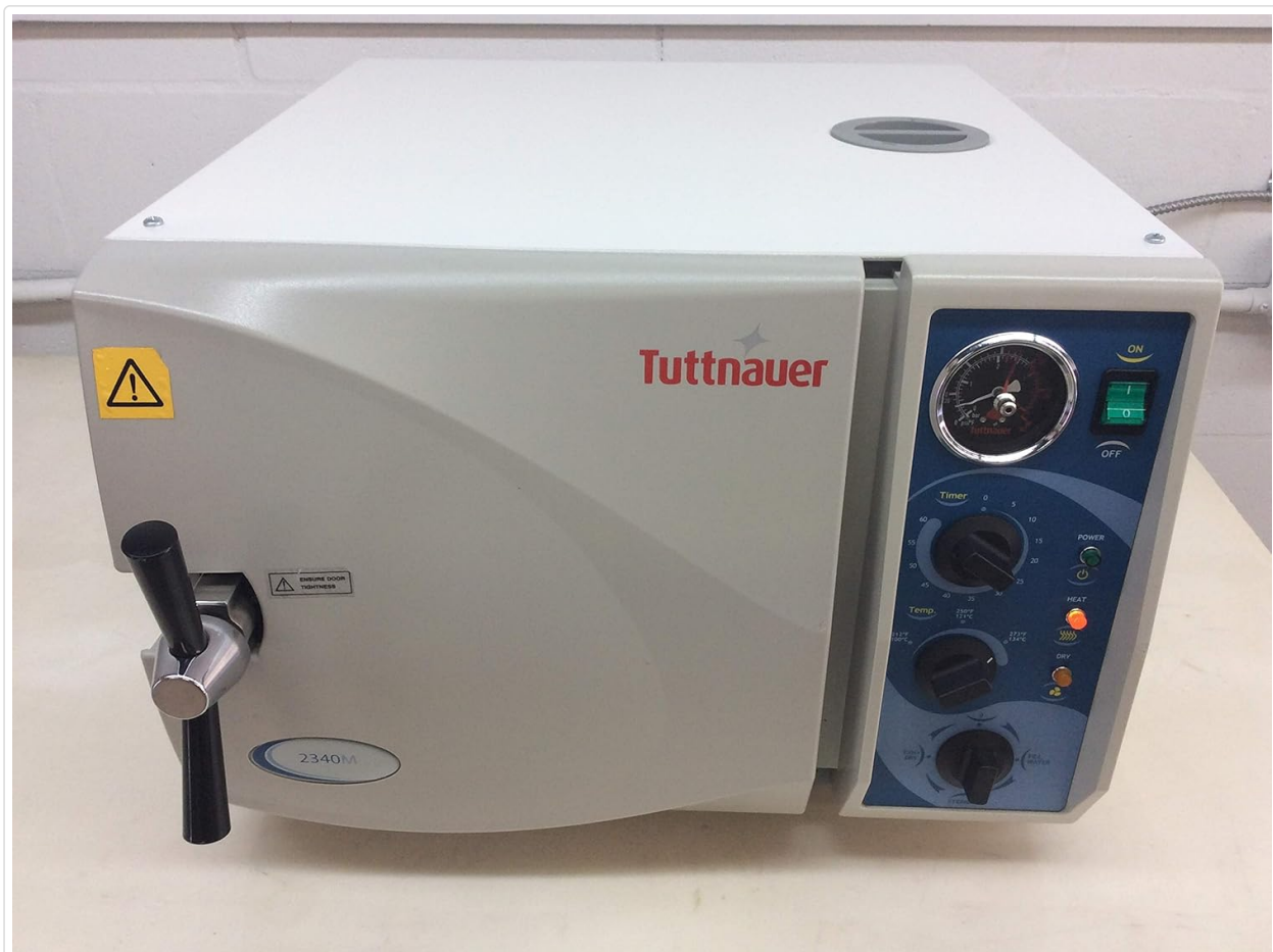
Figure 1: Front view of the Tuttnauer 2340M Manual Autoclave, showing the control panel and door handle.
