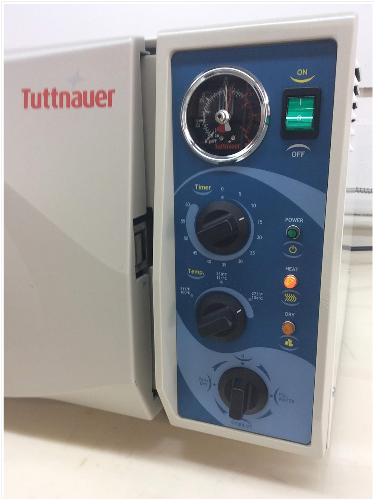
Figure 3: Detailed view of the control panel, highlighting the timer, temperature, and cycle indicator controls.
