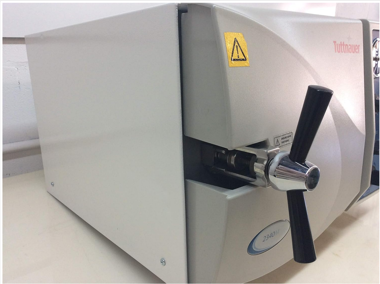
Figure 2: Side view of the autoclave, illustrating the robust door mechanism and handle.
