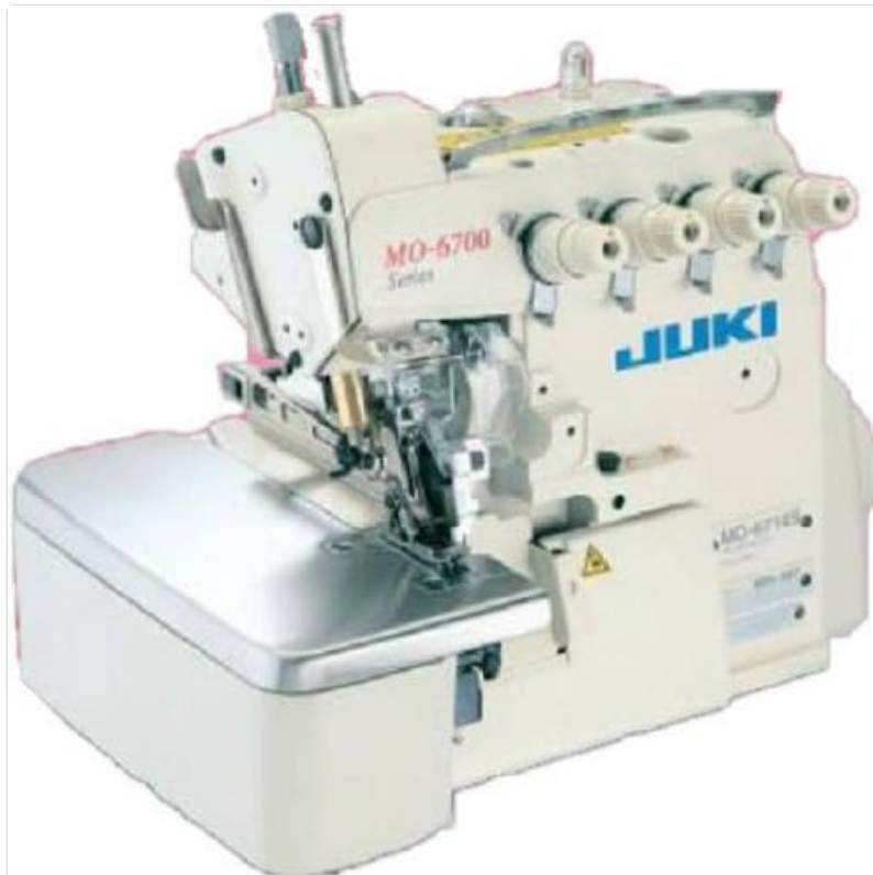
Figure 1: JUKI MO-6714S Industrial 4-Thread Overlock Sewing Machine. This image displays the complete machine, highlighting its white body, metallic work surface, and the four thread spools on top, along with the JUKI brand logo.
