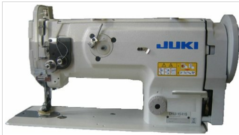
Figure 1: JUKI DNU-1541 Industrial Walking Foot Sewing Machine. This image displays the complete machine head, highlighting the needle area, thread tension assembly, and the JUKI branding.
