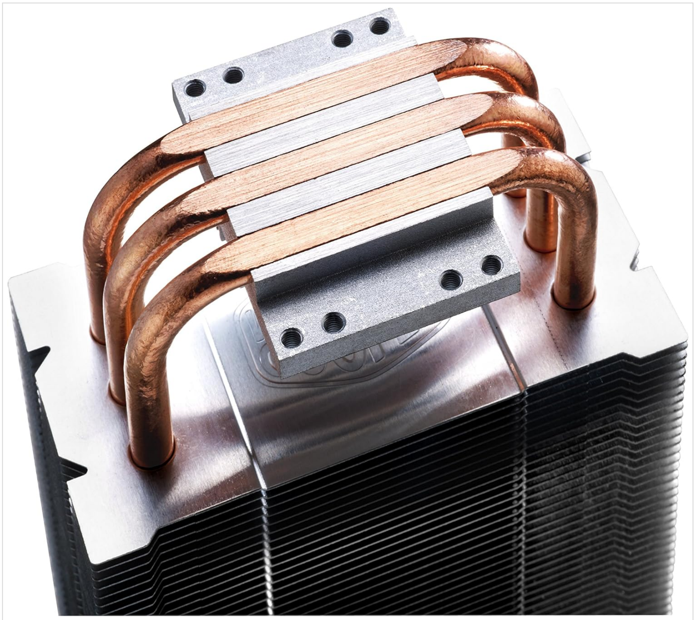
Figure 3.2: Close-up of the Hyper TX3's direct contact heat pipe base.
