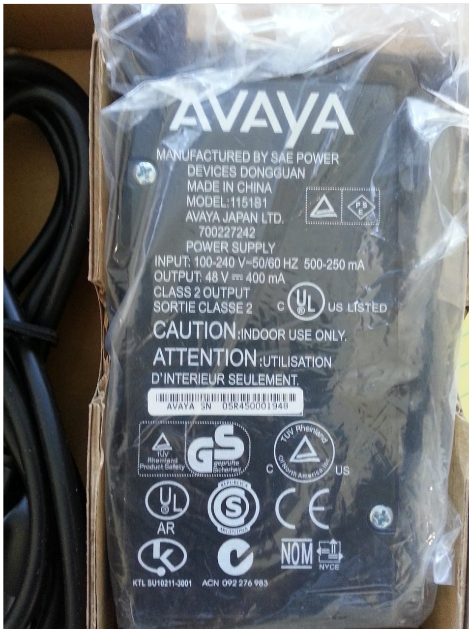
Image: Detailed label on the Avaya 1151B1 POE Power Supply Injector, displaying model number 1151B1, input specifications (100-240V, 50-60Hz, 500-250mA), and output specifications (+48V, 417mA). Various regulatory compliance marks are also visible.
