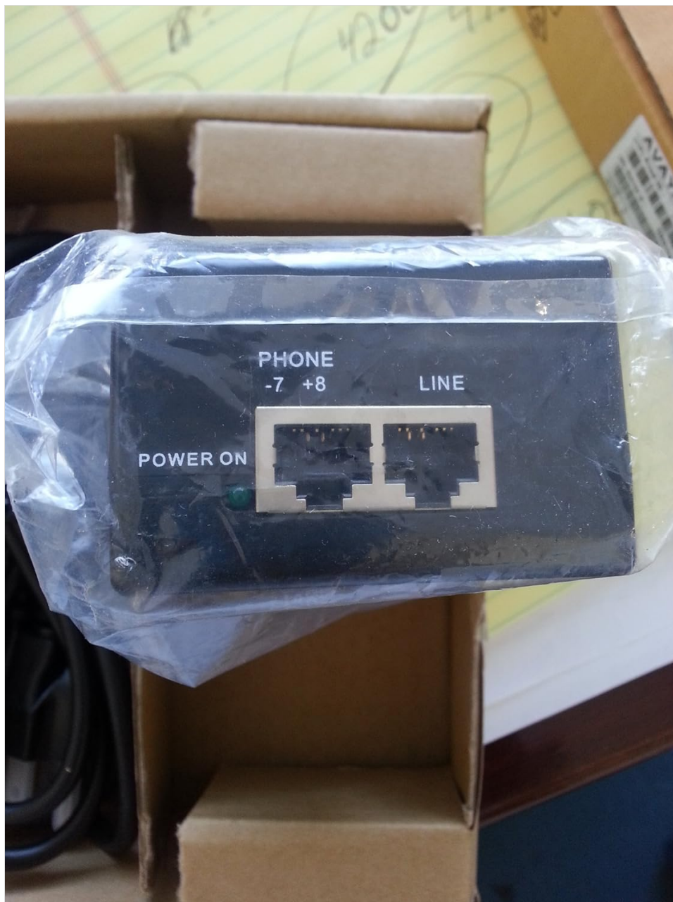
Image: Front view of the Avaya 1151B1 POE Power Supply Injector, showing two RJ45 ports labeled "PHONE" and "LINE", and a "POWER ON" LED indicator.
