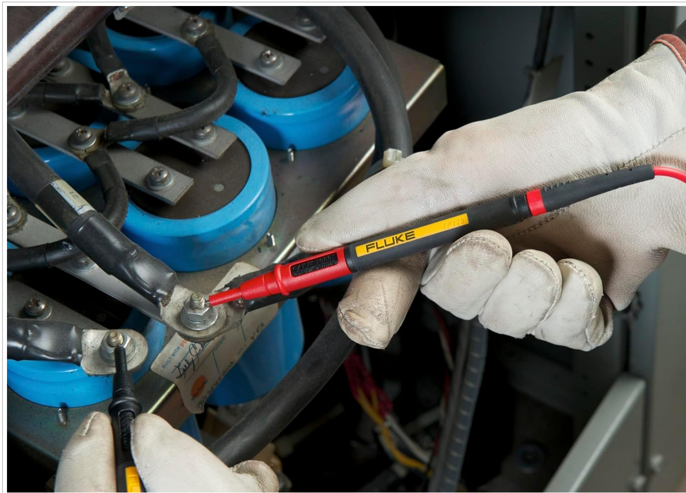
Figure 3: Proper use of the Fluke TP175 Test Probe for making a measurement on an electrical connection, demonstrating safe handling with gloves.
