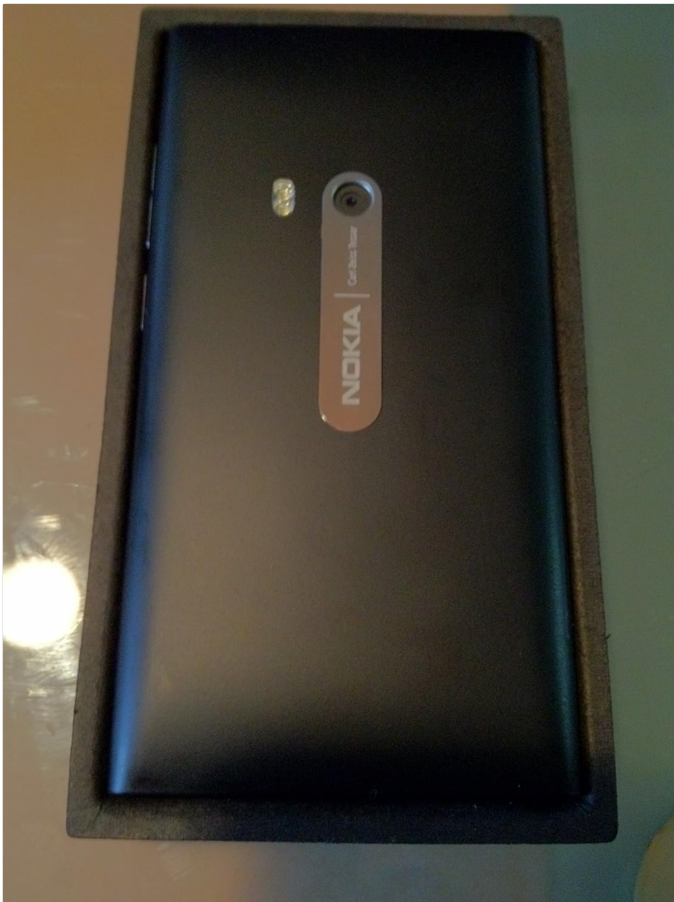
Figure 4.1: Rear view of the Nokia N9, showcasing the 8MP camera with Carl Zeiss optics.
