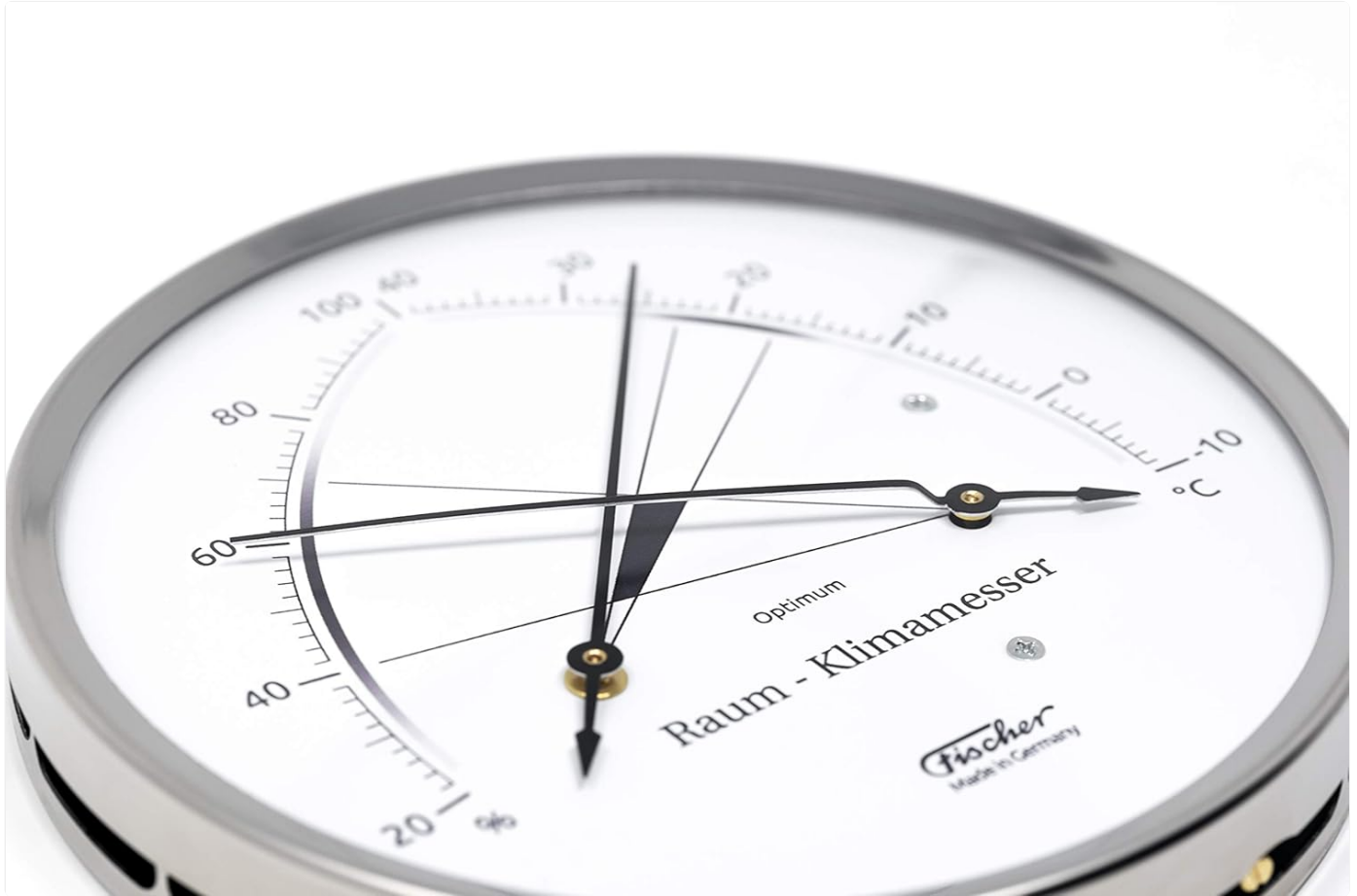
Figure 3: Close-up view of the dial, highlighting the temperature and humidity scales and the "Optimum" zone.
