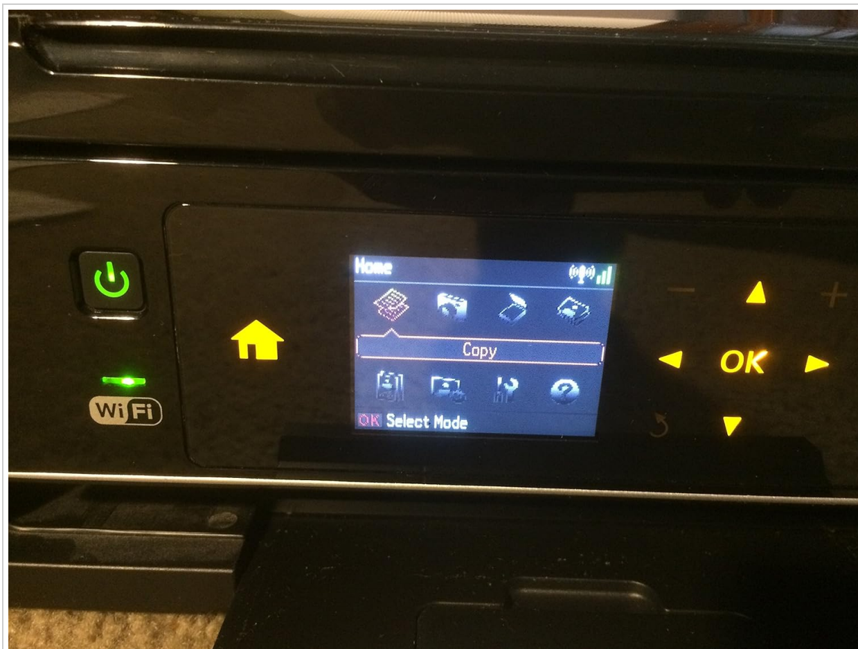
Figure 2.2: The printer's control panel, showing the LCD screen and navigation buttons.
