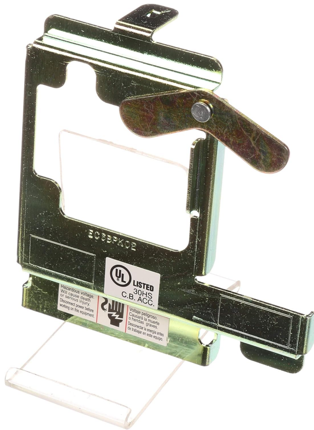
Image: Front view of the Siemens ECSBPK02 Mechanical Interlock, showing the metal bracket and the movable lever. This component ensures that only one of the two connected circuit breakers can be in the "ON" position at any given time.
