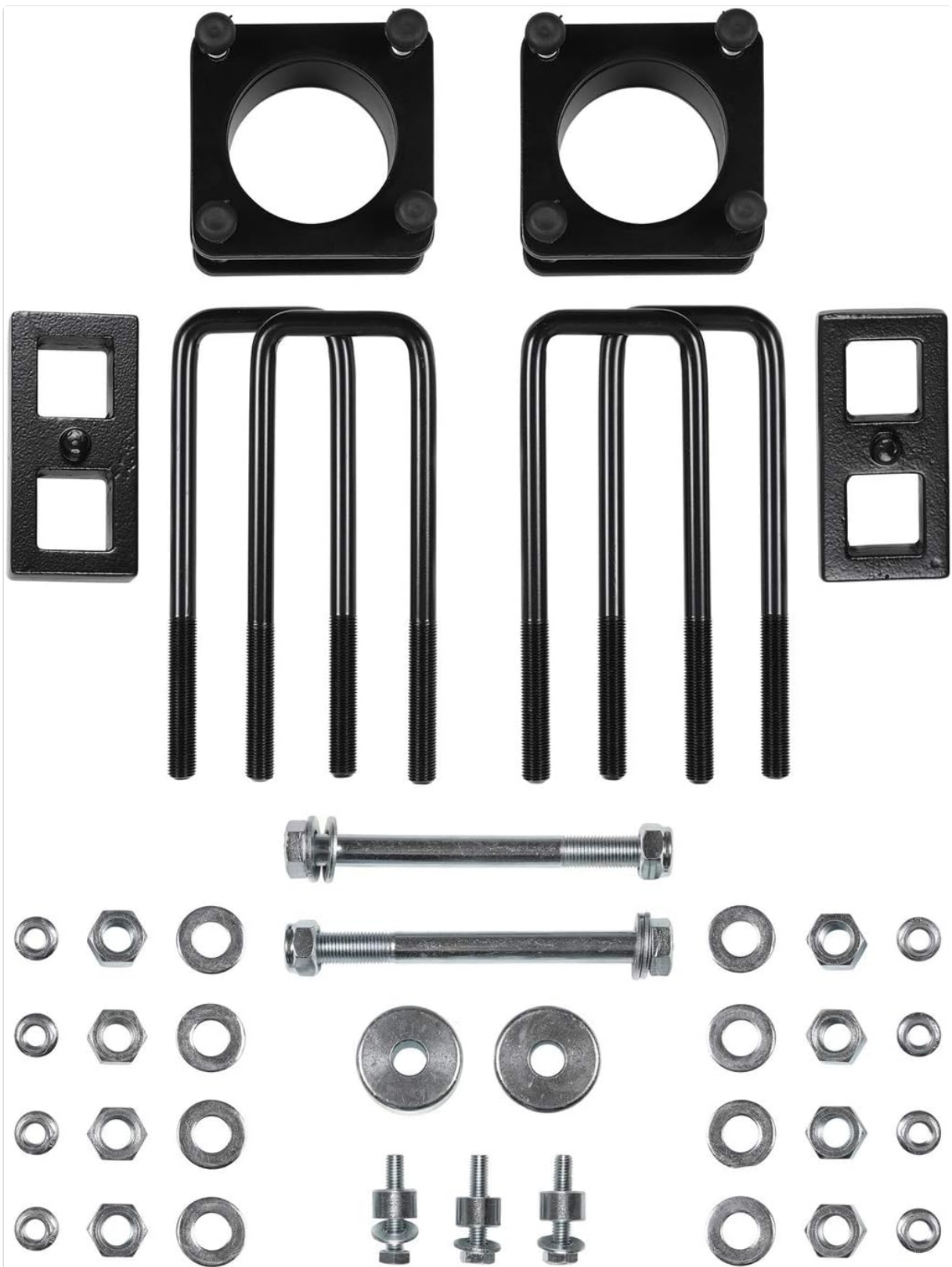
Figure 3.3: Complete set of components for the Pro Comp 65225K suspension lift kit, including front spacers, rear blocks, and hardware.
