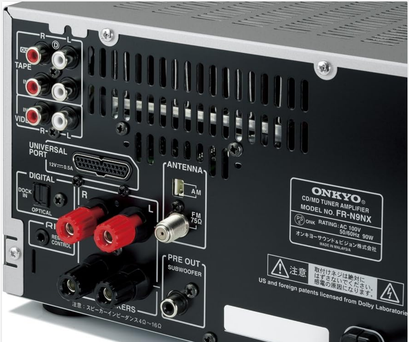
Image 1: Rear panel connections of the ONKYO FR-N9NX. This view highlights the speaker terminals (red and black posts), analog audio inputs (RCA jacks for TAPE IN/OUT, VIDEO IN, UNIVERSAL PORT), a digital optical input, and FM/AM antenna connections.
